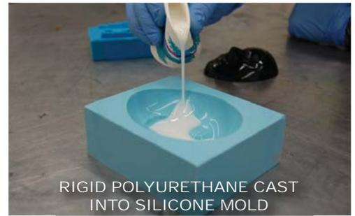
RIGID POLYURETHANE CAST INTO SILICONE MOLD
